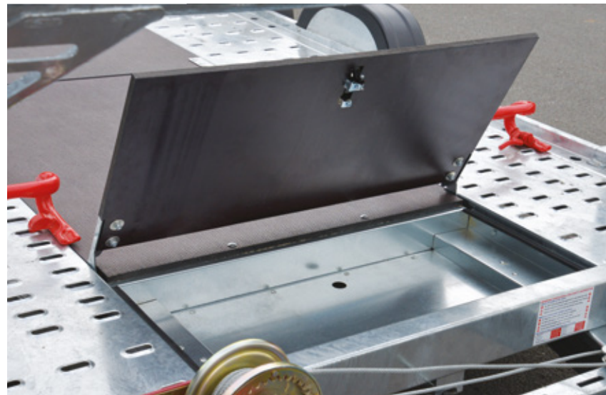
● Storage bed locker (front) Lockable front storage locker, with automatic lift lid.
